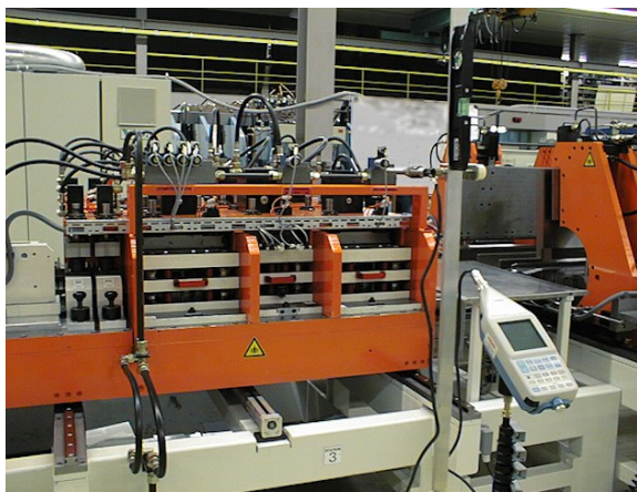
Emission measurement on a specified position at fixed distance and height
