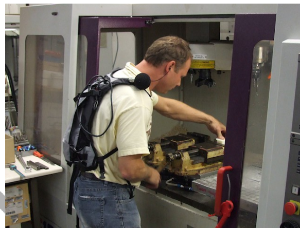
Exposure measurement: sound level meter is tied to the employee
